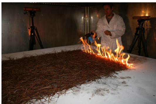
Fig. 4 Linear ignition for a 1 m × 1.5 m bed of Pinus pinaster needles inside the LSHR hood
